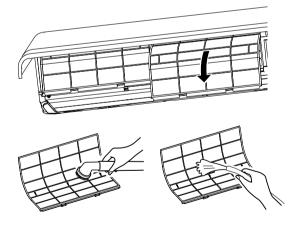
4. Insert the upper portion of air filter confirming to fit its right and left edges on the indoor unit until it is firmly set.
