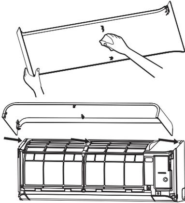
5. Check that the centre arm has been completely inserted and close the air inlet grille.
