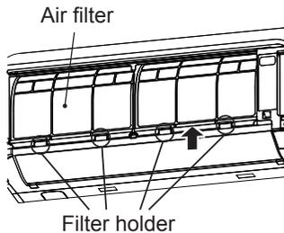
3. Use a vacuum cleaner to remove the dust from the filters or wash them with water.
