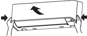
2. Take hold of the left and right handles of the air filter and lift it up slightly, then pull it downward to take it out from the filter holder.
