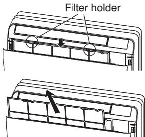
3. Use a vacuum cleaner to remove the dust from the filter or wash them with water. If you wash the air filter, dry them in the shade.
