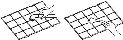
4. Insert the lower ribs of air filter into the slots then set it into the holding slot. (reverse the procedure number 2)
