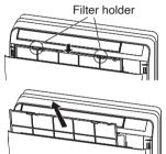
3. Use a vacuum cleaner to remove the dust from the filter or wash them with water. If you wash the air filter, dry them in the shade.
