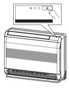
Continuous pressing of the 0 button for 10 seconds and above will start the forced cooling operation. (This will impose burden on the air conditioner. Do not perform this for the purposes other than test run.) In this time all indicators of indoor unit go on.
