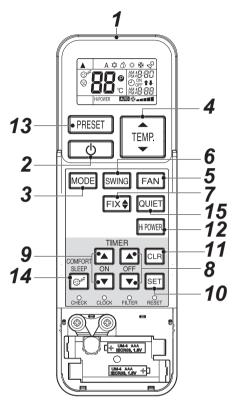
Infrared signal emitter 1 Transmits a signal to the indoor unit.
