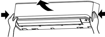
2. Take hold of the left and right handles of the air filter and lift it up slightly, then pull it downward to take it out from the filter holder.
