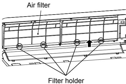
3. Use a vacuum cleaner to remove the dust from the filters or wash them with water.
